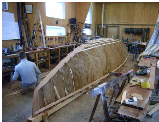
The keel and the frames are set for building the model which will receive the wooden layers (picture: A. Johnson)
